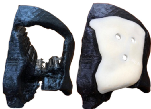
Fig. 16. Implant tests on the cranial model.
