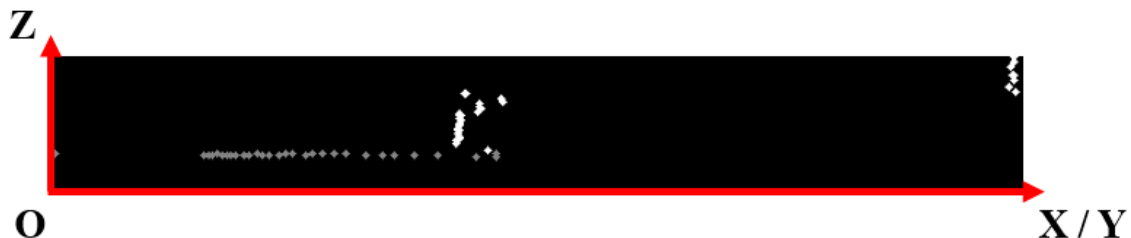
Figure 4. Side view of a channel. Detected ground points are colored with gray. X/Y means either the x-axis or the y-axis value is used, depending on the specific channel orientation.
