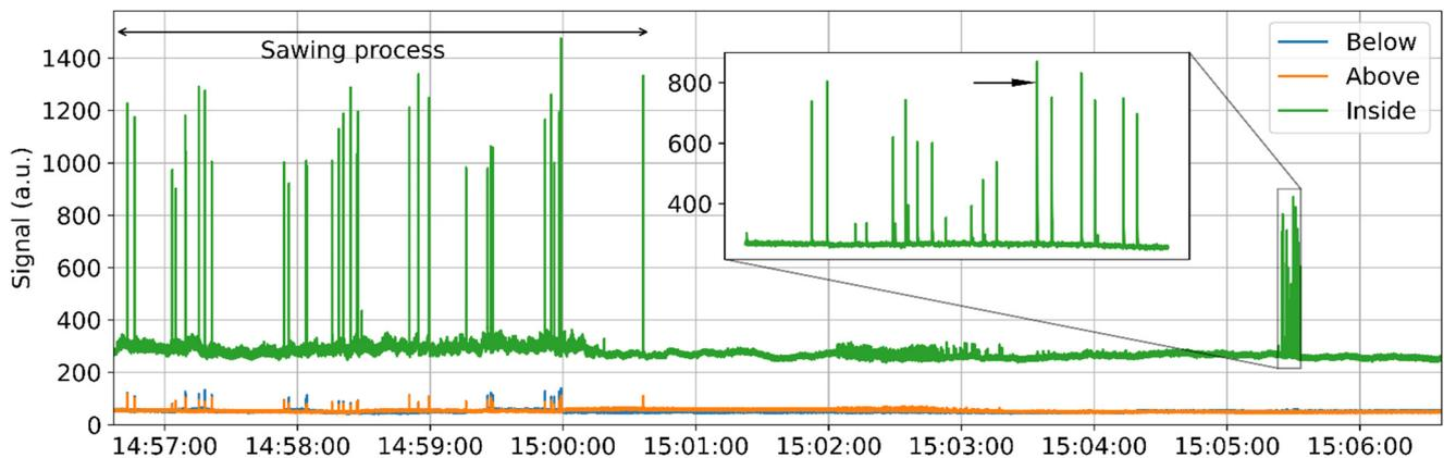
**Figure 7.** Temporal evolution of the summation result over the whole sensing section. The destructive testing process lasted ~4 min; then, an unexpected signal is detected, as shown in the inset.
