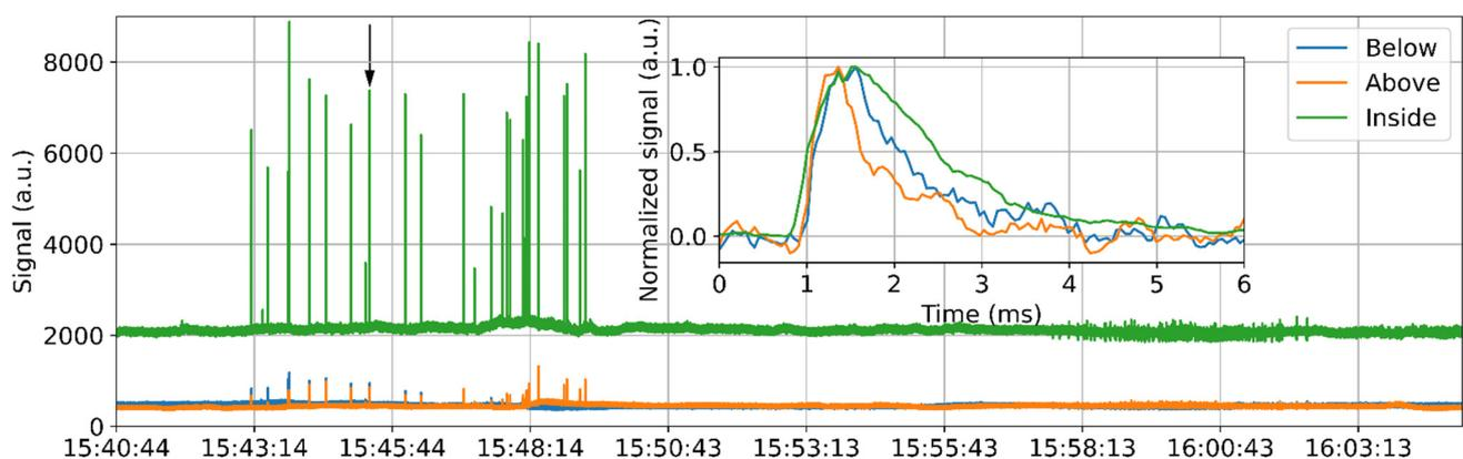
**Figure 6.** Temporal evolution of the summation result over the whole sensing section. Inset: zoom-in of one peak as indicated by the arrow; the DC level is removed and the peak is normalized to its maximum.
