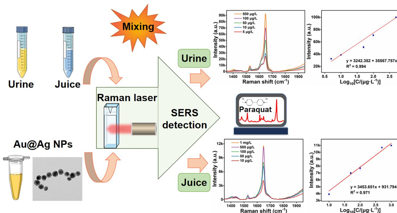
Figure 1. Scheme of the detection process using the POCT kit.
