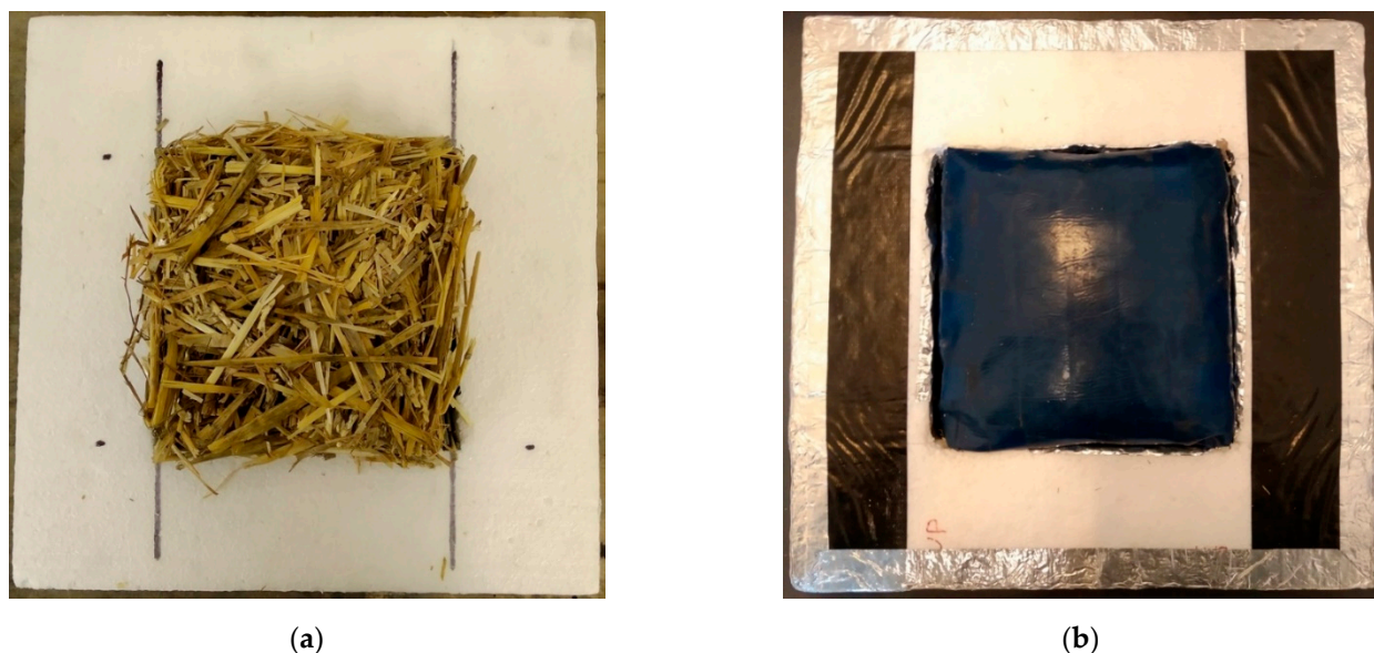
Figure 6. (a) Randomly oriented straw bulks; (b) closed measuring box filled with randomly oriented straw bulks.
