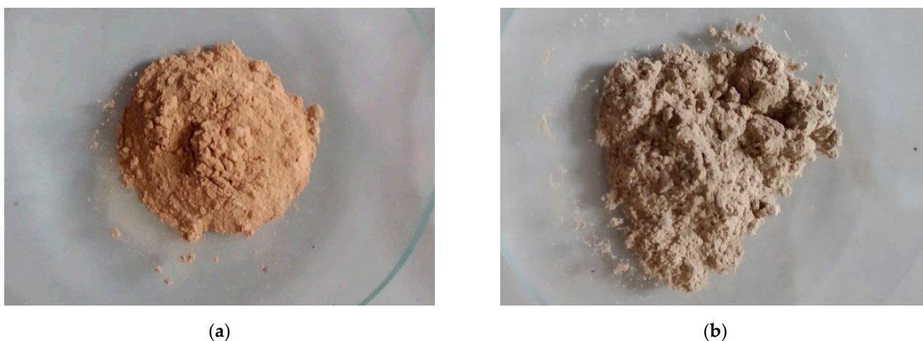
Figure 2. Milled straw dust of: (a) Type-1 straw; (b) Type-2 straw.
