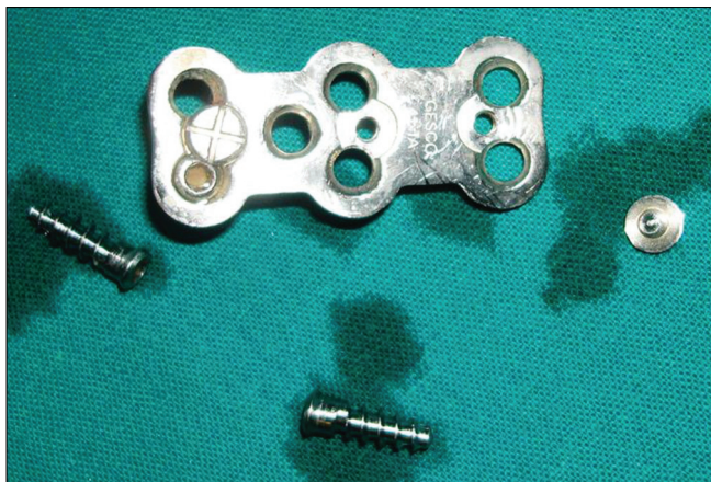
Figure 5: Plate and screws which were removed. The self-locking screw at upper end is still intact with one missed fixation screw. The lower locking and fixation screws are unscrewed
