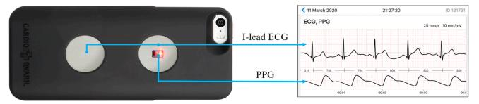
**Figure 1.** Characteristics of CardioQVARK device. On the **left side**, there is the electrode for I-lead ECG registration and on the **right side** the monitor for photoplethysmography PPG. The device is shown together with an example of the presentation of the recording.
