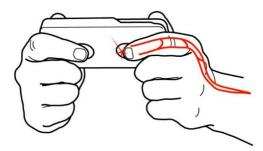
**Figure 2.** Recording of the ECG and the photoplethysmography image using the CardioQVARK<sup>®</sup> smartphone case. The index fingers are placed at the ECG electrode (left) and at the photoplethysmograph monitor (right).
