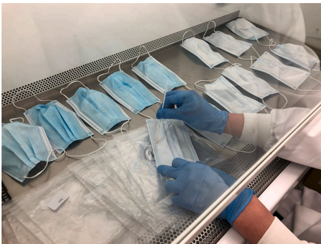
Fig. 2. Mask pooled swabbing process. For each batch of masks, the outer (EXTERNAL) surfaces were all swabbed with one swab to pool any potential viral RNA to enhance the sensitivity of the detection. A similar process was repeated for the inner (INTERNAL) surface of the masks.
