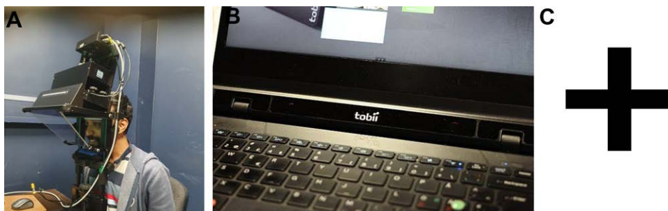
Fig.1. Common elements utilized within eye-tracking studies. Different models of eye-trackers (A and B) and an example of a fixation cross (C). A, A participant using a model of eye-tracker (Eyelink 1000) that is mounted away and in front of a monitor. B, A screen-mounted eye-tracking device (Tobii Pro Nano). C, An example of a typical fixation cross that directs the attention of a participant to a specific point on the screen.
