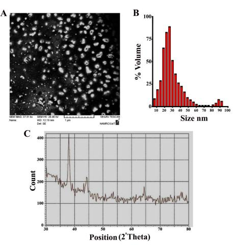
Figure 2. Morphological and structural characteristics of AgNPs. (A) SEM image. (B) DLS. (C) XRD pattern.
