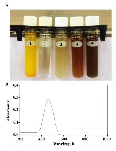
**Figure 1.** Formation of AgNPs. (**A**) Color changes: 1, *Annona muricata* peel extract; 2, silver nitrate solution; 3, silver nanoparticles at a concentration of 1 mM of AgNO<sub>3</sub>; 4, silver nanoparticles at a concentration of 2.5 mM of AgNO<sub>3</sub>; and 5, silver nanoparticles at a concentration of 5 mM of AgNO<sub>3</sub>. (**B**) UV-spectroscopy of AgNPs.
