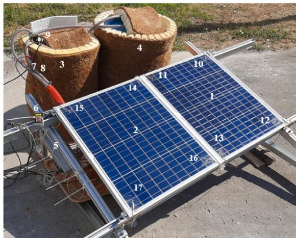
**Fig. 1.** Experimental setup (1) reference PV module, (2) PV/T system, (3) nanofluid tank, (4) water tank, (5) data logger, (6) solar radiation sensor, (7) inlet, (8) outlet, (9) flow sensor, (10–17) thermocouples.
