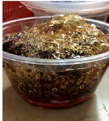
Figure 5. Sample of phenol formaldehyde (PF) resin prepared at 100 °C.
