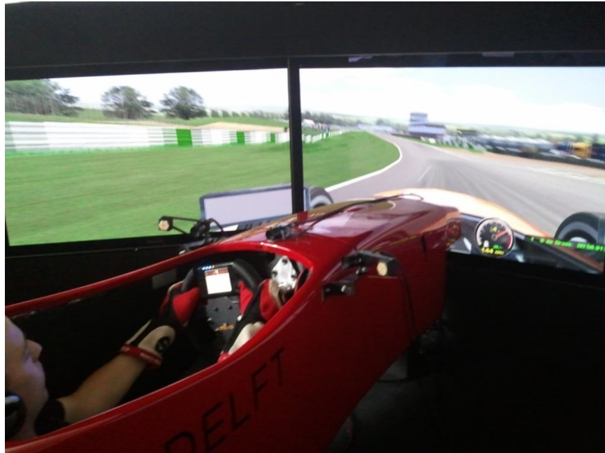
Fig 1. Overview of the racing simulator and eye tracker.
