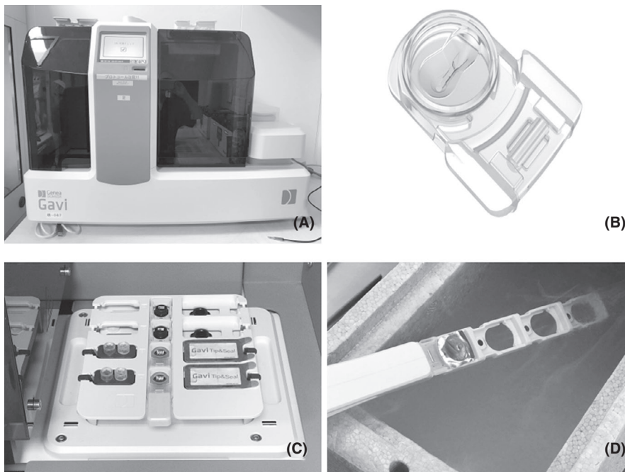
FIGURE 1 Images of the Gavi system and its consumable components. A, Appearance of the whole Gavi system with the automated pipette inside. B, Gavi pod, which can preserve oocyte, embryo, and blastocyst on a slit in the pod. C, Vitrification media, cassette, and disposable tip and seal. D, After the dehydration step, the Gavi pod is dumped into liquid nitrogen to complete the vitrification step
