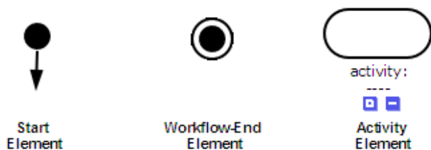
Figure 3 Graphical notation of Workflow elements available in WebWFlow. BioWMS has three main elements: 1) Workflow-Start element; 2) Workflow-Stop element; 3) Workflow-Activity element.
