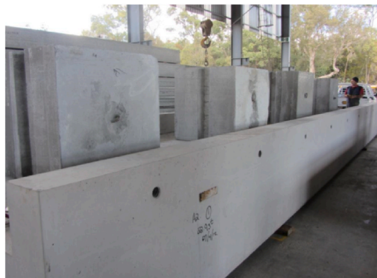
Fig. 14. Precast fly ash and slag alkali-activated floor beams used in the GCI building in Australia [149].
