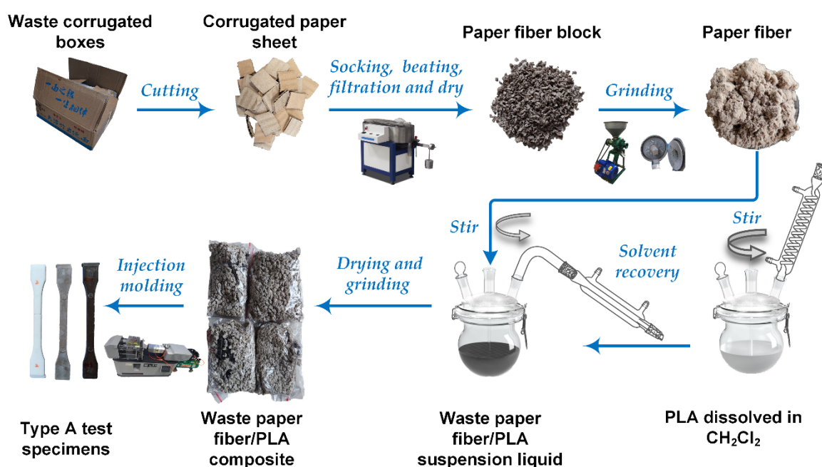
Figure 1. Preparation process diagram of the WCPF/PLA composite.
