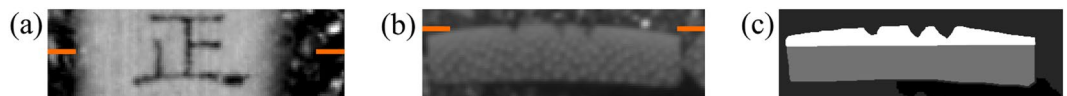
Figure 7. (a) Randomly selected carving slice of an extracted slip. At the position of the orange lines, a depth view was extracted shown in (b). The depth view shows the slip surrounded by air and soil. The segmentation map is shown in (c). Recto layer (white), verso layer (light gray), soil (dark gray) and air (black) were manually segmented. An analysis of the mean intensities of the areas reveals that the recto layer's attenuation differs by 29% from the soil's one.
