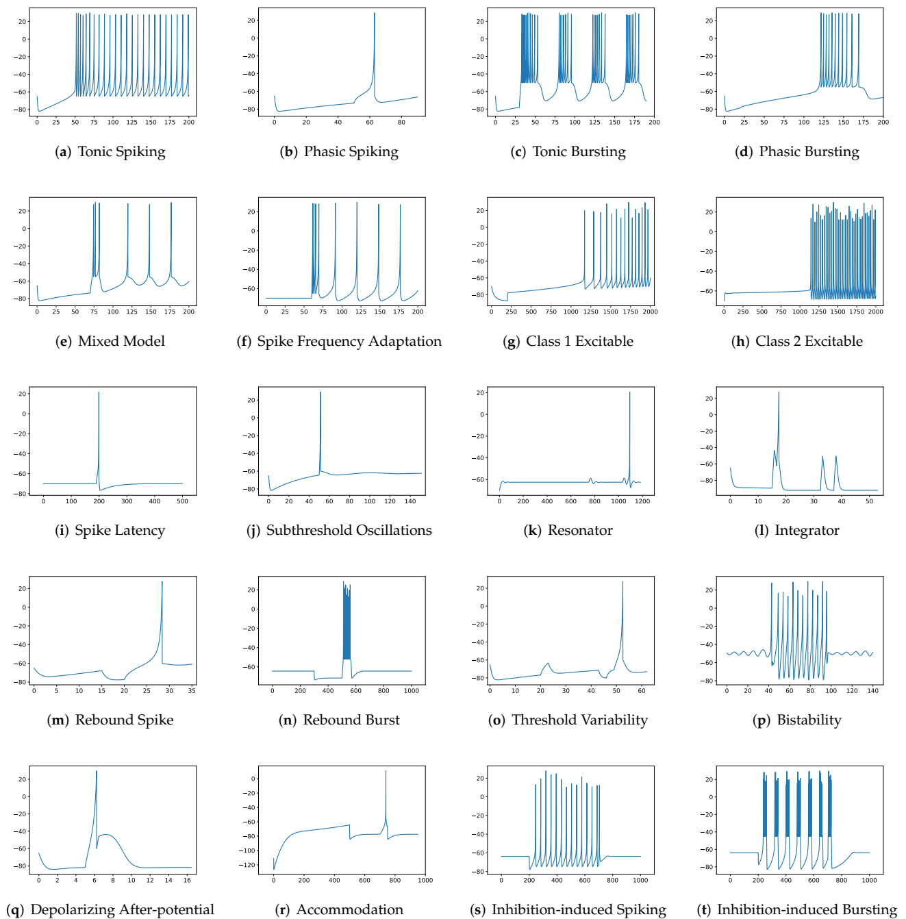
Figure 1. Twenty firing behaviors generated by the Izhikevich Model, where y-axis is the membrane potential (mV) and x-axis is the time (ms).
