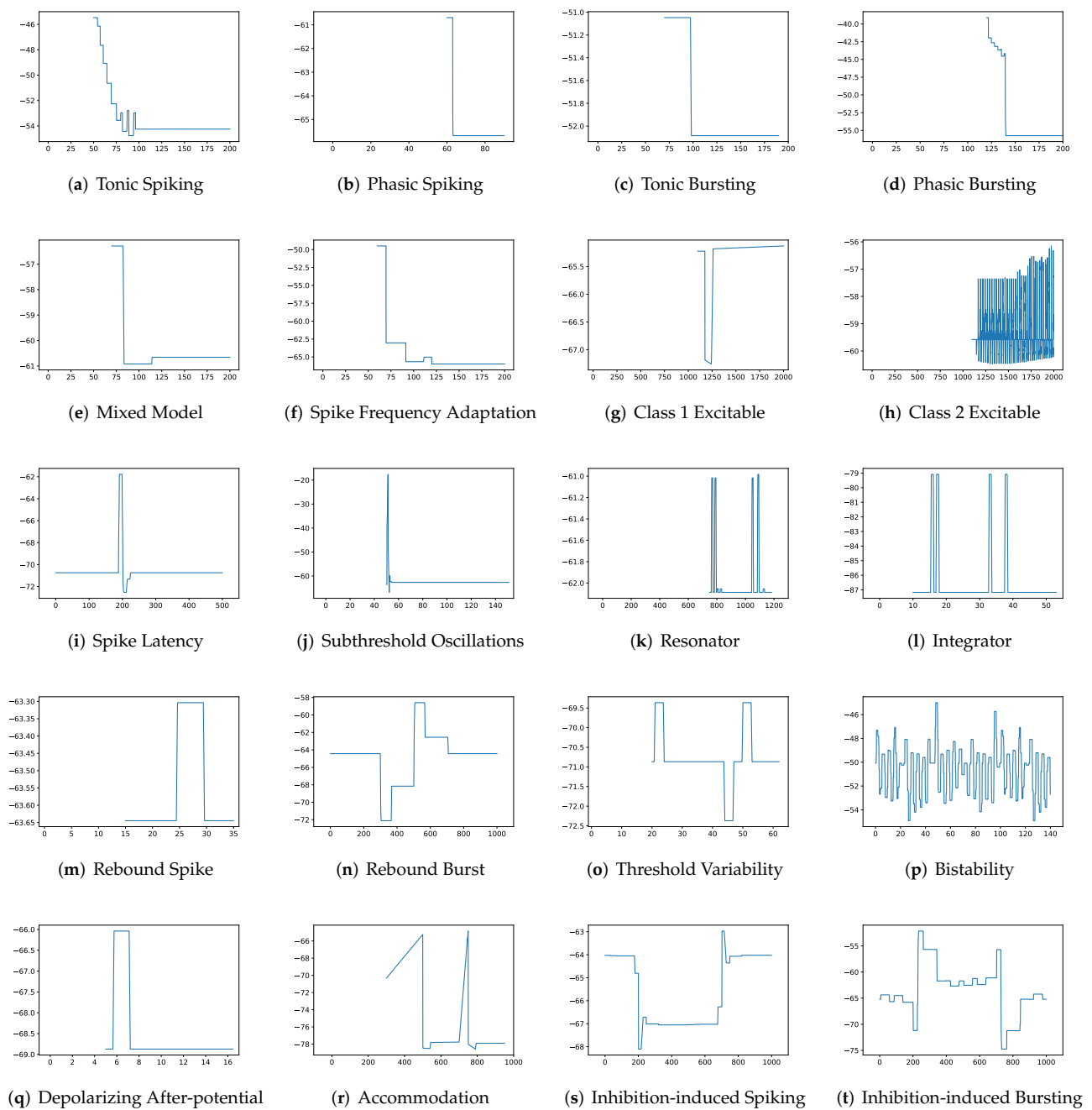
Figure 7. Membrane potentials of RSRM, where y-axis is the membrane potential (mV) and x-axis is the time (ms).
