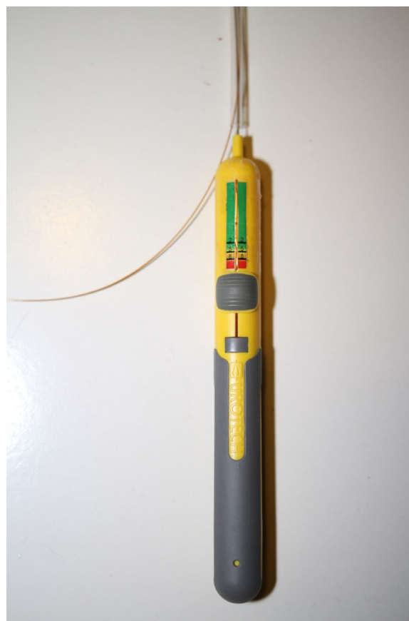
Fig. 1 A handle with a new colored millimeter scale and slider
