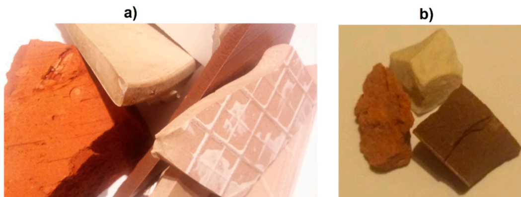
Figure 5. Close-up of the surface of the ceramic: (a) in the form of waste, (b) a form representative of the shape of aggregate grains.
