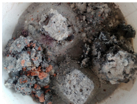
Figure 11. Samples of composites after 240 days of saturation in the solution.
