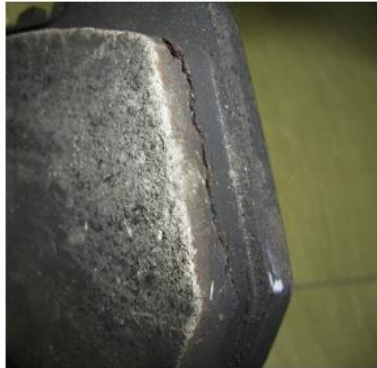
Figure 8. An example of a “distorted” disk brake pad as a result of high temperature and excessive load (reprinted/adapted with permission from ref. [13]. 2022, Elsevier).
