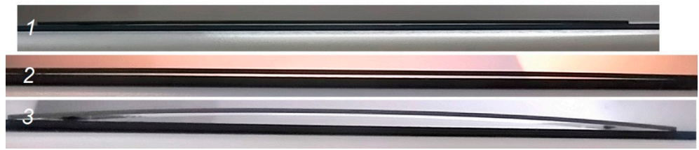
Figure 4. Side view of substrates: 1—initial anode substrate; 2—after YSZ electrolyte film deposition, 3—after 1200 °C annealing; YSZ electrolyte is deposited on top.
