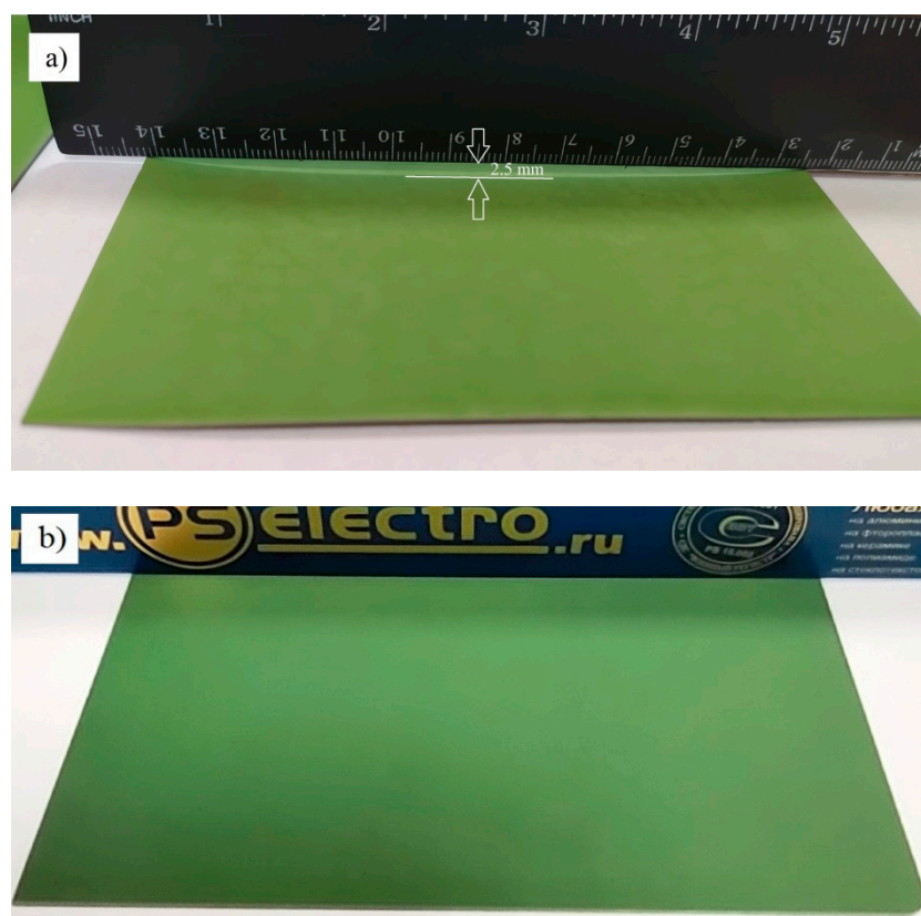
Figure 11. Photographs of ASCs with YSZ electrolyte film deposition: (a) in oxide mode followed by stress-free annealing; electrolyte on ASC underside, (b) in transition mode and annealed under load; electrolyte on ASC top.
