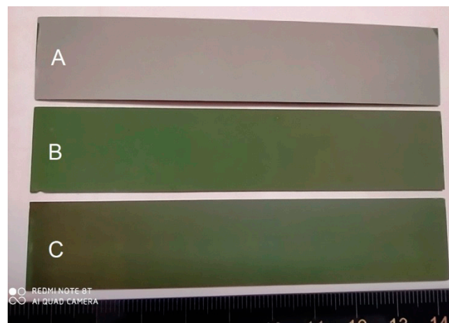
Figure 5. Photograph of YSZ electrolyte films (from Table 1) annealed at 1200 °C: A —film 3, B —film 2, C —film 1.
