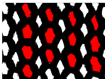
Figure 13. Measurement of the stitch size of the ground fabric.
