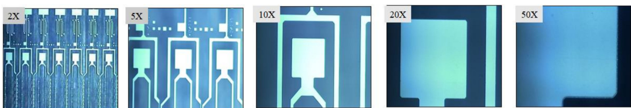
Figure 12. Various magnification lens with 2 \times , 5 \times , 10 \times , 20 \times , and 50 \times are illustrated by area-CCD.
