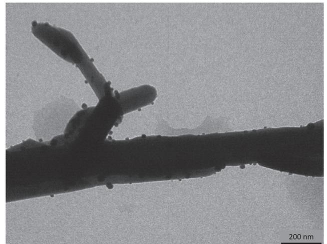
**Fig. 1.** Photomicrograph of vanadate nanowires and silver nanoparticles of AgVO<sub>3</sub>.
