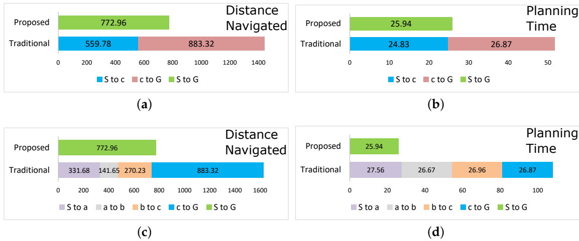
Figure 5. Comparison of proposed vs. traditional method. (a,b) Distance and time with one obstacle c in Figure 4d,e vs. Figure 4f; (c,d) Distance and time with three obstacles a–c in Figure 4.
