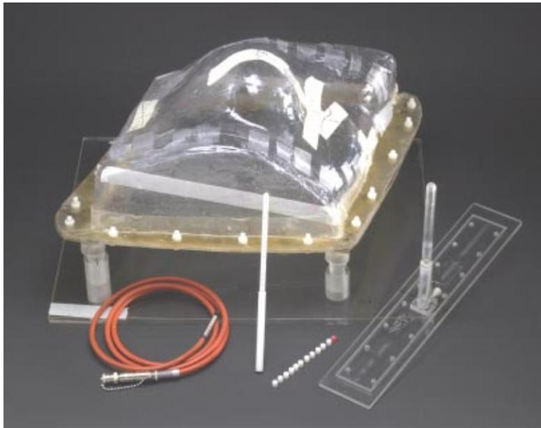
FIG. 1. (Color) The anthropomorphic breast phantom, ion-chamber sleeve, and chamber localization device and spacers are shown, as well as the waterproof PTW ion chamber used for measurements. The superior and lateral portions of the phantom are shown on the top and right sides of the figure, respectively.
