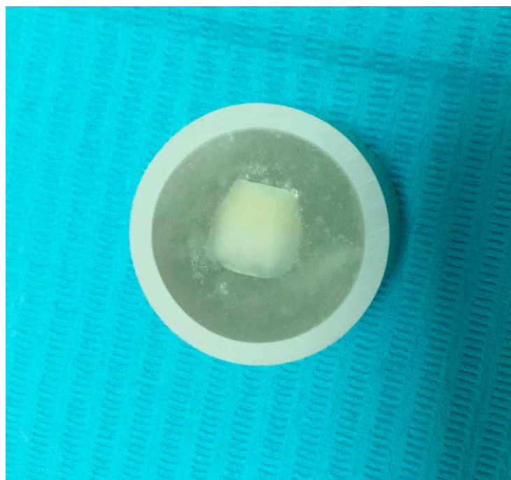
Figure 1. Embedded teeth sample in acrylic resin.
