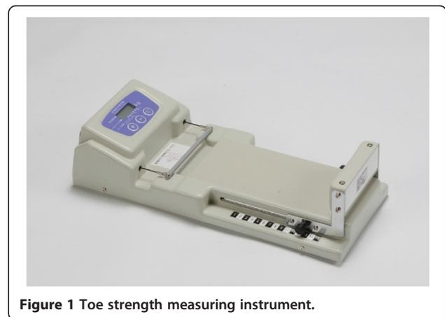
Figure 1 Toe strength measuring instrument.
