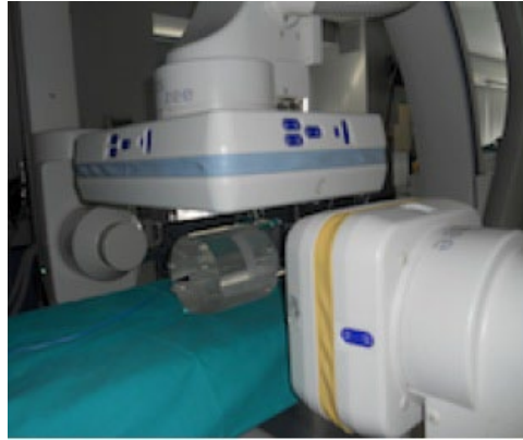
FIG. 4. Biplane acquisition setup using CT head phantom.
