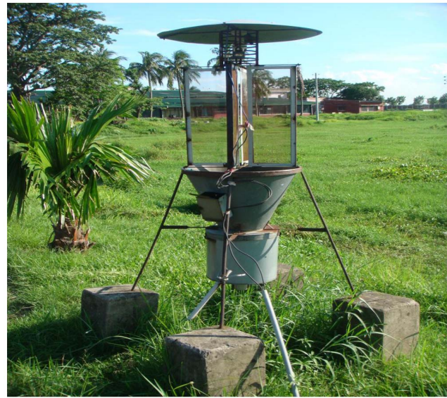
Figure 1. The light trap used to collect brown planthopper (BPH) in this study. It was placed adjacent to a rice field belonging to Bangladesh Rice Research Institute (BRRI). doi:10.1371/journal.pone.0091678.g001
