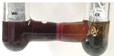
Figure 7. H-tube used for electrodeposition under inert conditions. A potential of -3.7 V was applied for 16 h to a solution of tellurium in [P_{66614}][OAc] at 100^\circ\text{C} . The current was about 0.4 mA. A greyish powder of tellurium formed in both electrode compartments. The solution at the working electrode (WE) is still intensely colored purple, while the solution at the counter electrode (CE) has turned translucent brown.
