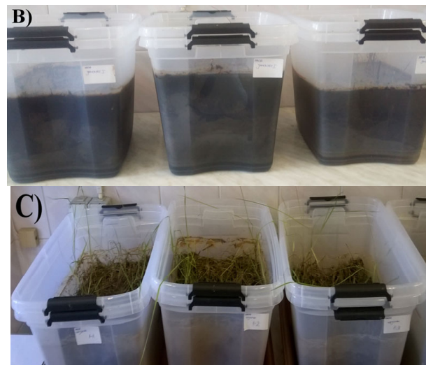
Figure 2. (A) Experiment scheme; (B) containers with flooded soil (7 days of flooding); (C) containers with drained soil (56 days after the floods ended) (author's materials).
