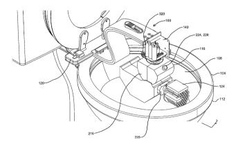
Fig.11 Giddel robot attached to toilet commode (D'Souza et al. 2019)
