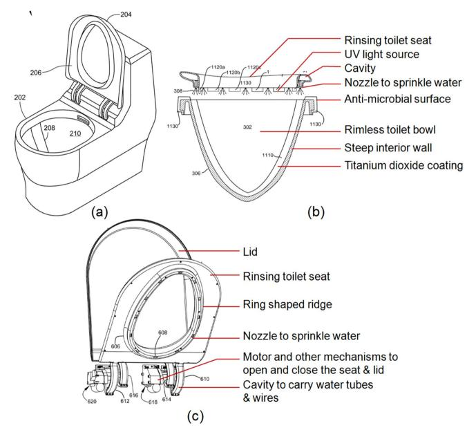
Fig. 9 a Design of an antimicrobial self-cleaning toilet proposed by Hall et al. b Rinsing seat with nozzles and UV source placed above rimless bowl and c Lid and rinsing seat arrangement (Hall et al. 2018)
