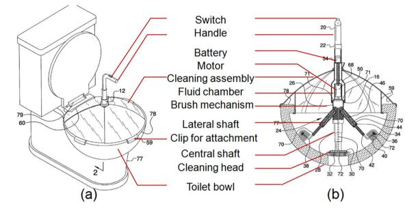
Fig. 7 a Toilet bowl cleaning assembly designed by Ba-Akeel et al. attached onto a toilet bowl; b Cross-sectional view of the toilet bowl cleaning assembly (Ba-Akeel and Ghaemi 2011)
