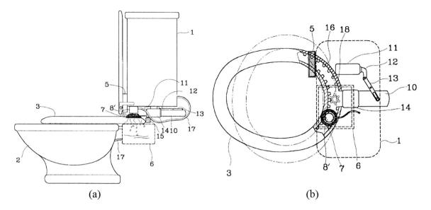
Fig. 2 Design of toilet cleaning system as proposed by Yu a side view; b top view; (Yu 1998)
