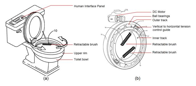
Fig. 8 a Design of the device proposed by Qualls et al. to automatically clean a toilet bowl; b A cross-sectional perspective top view under the rim (Qualls and Jones 2017)
