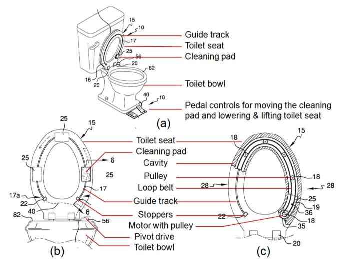
Fig. 5 a Design of toilet cleaning apparatus proposed by Graves et al.; b bottom view of the toilet seat while the seat is lifted; c partial cross sectional view of bottom part of toilet seat while seat is lifted (Graves and Graves 2009)
