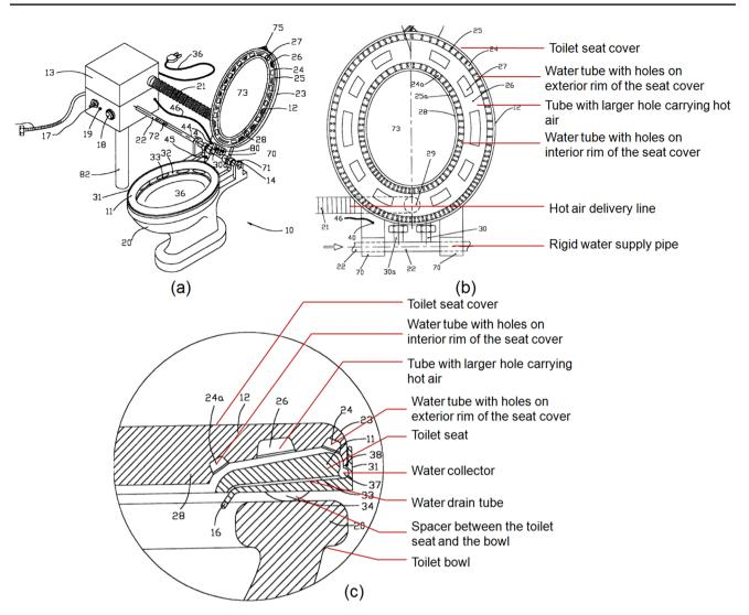
Fig. 3 a Design of automatic toilet cleaning apparatus invented by Sadegh et al.; b bottom view of the toilet seat cover; c Enlarged section of the outer edge of the toilet seat in closed position (Sadegh et al. 1999)
