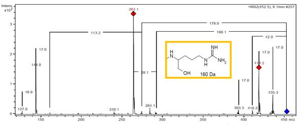
**Figure 5.**  $MS_2$  fragmentation pattern of the protonated from of the 15N-labeled new peptide aldehyde compound (452 m/z) after reduction by NaBH4. m/z= Mass-to-charge ratios. The intensity of the ion on the y-axis is given as counted ions per second (cps) and the mass-to-charge ratio (m/z) on the x-axis.
