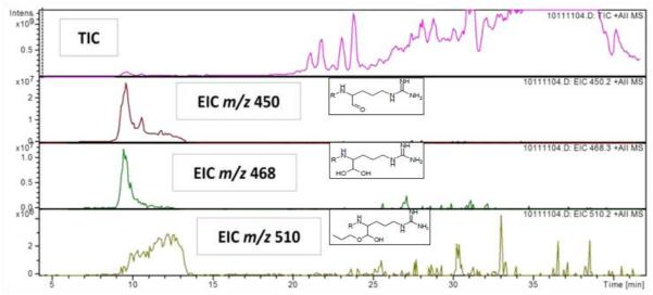
Figure 3. Total ion chromatogarm (TIC) and extracted ion chromatogarm (EIC) of the protonated  $[MH^+]$  new peptide aldehyde compound (450.2 m/z),  $[M + H_2O + H^+]$  (468 m/z) and  $[M + IPA + H^+]$  (510.2 m/z). The x-axis represents retention time (min), and the y-axis represents signal intensity. Intensity is measured in counts per second (cps).
