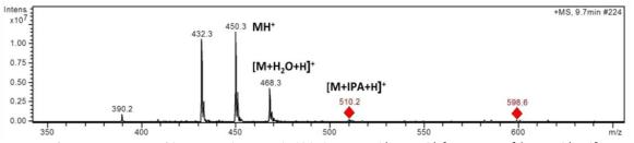
**Figure 2.** +MS fragmentation patterns of the protonated new peptide aldehyde compound (450.3 m/z),  $[M + H_2O + H^+]$  (468.3 m/z) and  $[M + IPA + H^+]$  (510.2 m/z). m/z= Mass-to-charge ratios, The intensity of the ion on the y-axis is given as counted ions per second (cps) and the mass-to-charge ratio (m/z) on the x-axis.
