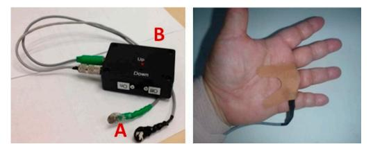
**Figure 7.** The stimulation device and the "puck". A: small vibrating disks which are taped to the skin over proprioceptive fibers as in the figure on the right on the hand (or foot), B: a stimulation device, containing a low voltage battery that powers the vibration motor through flexible cables. https://journals.plos.org/plosone/article?id=10.1371/journal.pone.0157349 (accessed on 6 February 2021).
