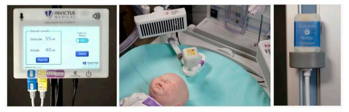
**Figure 1.** Neoasis<sup>™</sup> system: on the left is the control unit with the external noise sensor, in the center are the speakers and the internal noise sensor, on the right is the additional "outside" noise sensor. http://www.invictusmed.com/neoasis/ (accessed on 6 February 2021).
