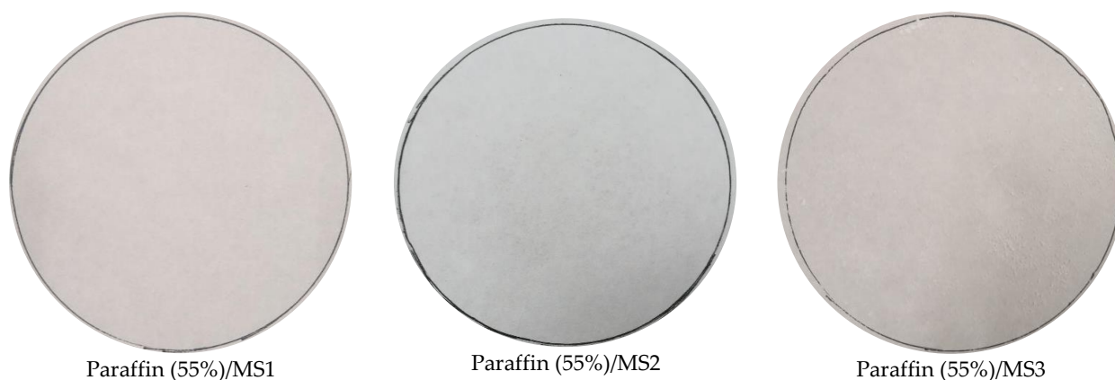
Figure 2. Leakage test of MS1, MS2 and MS3 SS-PCMs with different paraffin mass proportion after heating.
