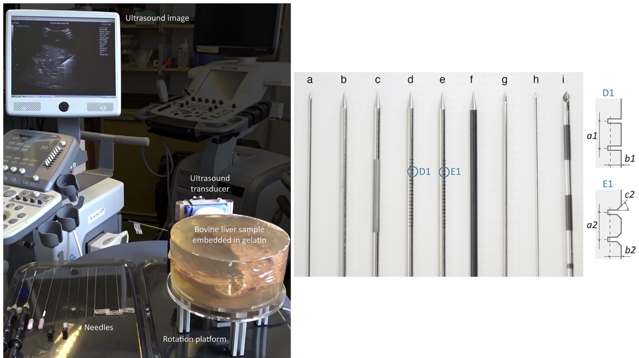
FIGURE 1 Experimental set-up with an ex vivo model of bovine liver and the set of percutaneous needles used. The overview of the set-up shows the liver sample, US transducer and US machine, as well as the needles used, including: (a) polished stainless steel (1 mm), (b) polished stainless steel (2 mm), (c) sand-blasted stainless steel (2 mm), (d) EDM stainless steel I (2 mm), (e) EDM stainless steel II (2 mm), (f) nitinol (2 mm), (g) trocar (18G), (h) chiba (22G), and (i) RFA (2 mm) needles. The kerfed needles are shown in a cross-sectional view, D1 and E1, where a1 = a2 = 1 mm, b1 = b2 = 0.5 mm, and c2 = 45^\circ \times 0.2 mm
