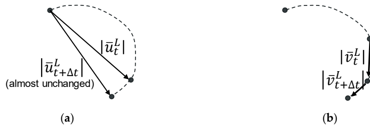
Figure 7. Displacement and velocity vectors of a moving point in image coordinate. The norm of the displacement vector does not represent the movement, making displacement an inappropriate indicator for synchronization. (a) Displacement vector history. (b) Velocity vector history.
