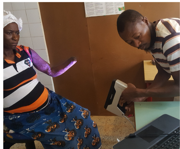
Figure 1. The scanning process. This figure shows the local physiotherapist scanning the dimensions of the residual limb of a patient.
