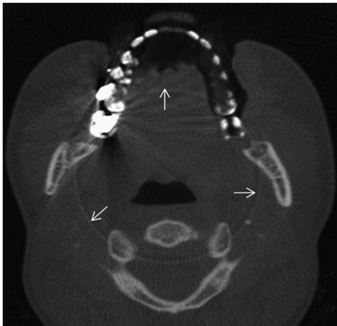
Figure 4: Ring artifact caused by calibration error
