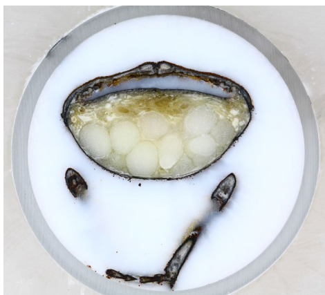
Figure 8. Beetle surface image after micro-milling. Notice intact eggs and chitin structure.
