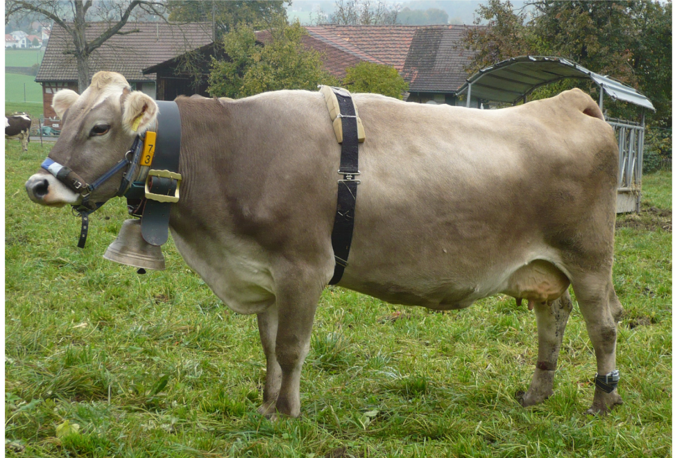
Fig 1. Experimental cow wearing a bell and measuring equipment. A thorax belt for measuring heart rate variability, a halter for recording feeding, ruminating, and head movements, and a 3D accelerometer at the hind leg for recording activity and lying were used for data recording after 24 hours of habituation.
