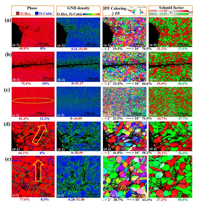
the local microstructure evolutions caused by shearing lead to dynamic recrystallizations and play an important role of softening during severe plastic deformation.
