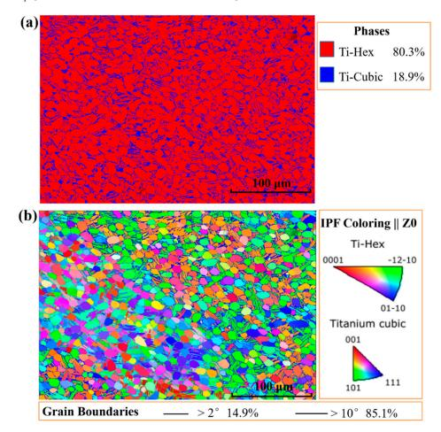
**Figure 1.** The electron backscattered diffraction (EBSD) analysis of the as-received dual-phase Ti alloy, (**a**) phase map; (**b**) the coupling analysis of inverse pole figure and the grain boundary map.
