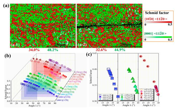
**Figure 6.** The theoretical Schmid factors (SFs) referring to experimental observations: (**a**) experimental characterizations of SFs of the left and the right side of the hat-shaped specimen; (**b**,**c**) 3D and 2D views of the theoretical SFs.
