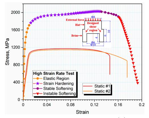
**Figure 2.** The stress–strain of dual-phase Ti alloy at the strain rate of  $1.8 \times 10^4 \text{ s}^{-1}$  and the static one (0.001 s<sup>-1</sup>) together with the geometry of the hat-shaped specimen.
