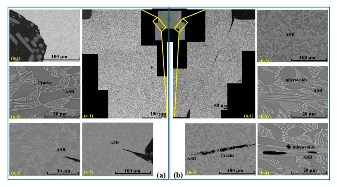
**Figure 3.** The multi-scale SEM characterizations of adiabatic shear bands in the hat-shaped specimen. The left part and the right part of the weak areas in the hat-shaped specimen are marked by yellow frames in (**a-1**) and (**b-1**), respectively. (**a-2**)~(**a-5**) reflect the typical features of the selected right region, such as ASB, microvoids and  $\alpha+\beta$  phases, while the selected left region is identified in (**b-2**)~(**b-5**).
