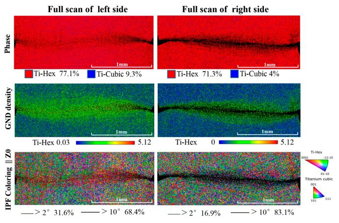
**Figure 4.** The EBSD features of the hat-shaped specimens in terms of phase map (Ph), geometrically necessary dislocation (GND) map, and the coupling analysis of inverse pole figure and grain boundary map (IPF+GB).
