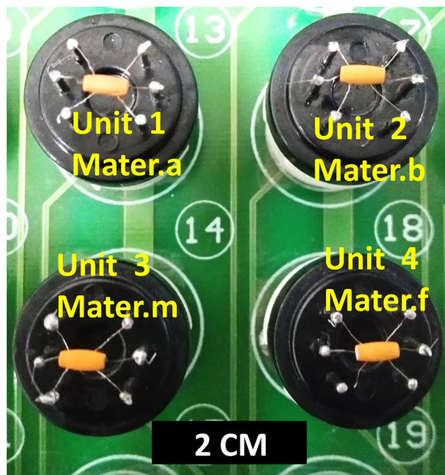
Figure 1. Photograph of the sensor array. Each unit in the array is a heater-type sensor. The black scale bar represents 2 cm.
