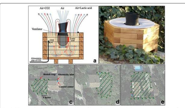
Fig. 2 Biobelt traps installation in the treated houses. a Scheme of the trap function, based on the Biogents mosquito traps. b Photo of an individual trap. c-e Spatial schematic depiction of the array of the "belt" of traps around three treated houses, prospected in the area Modulestraps are shown in green, control center in blue and electricity inlet in red. The area protected by the barrier is hatched
