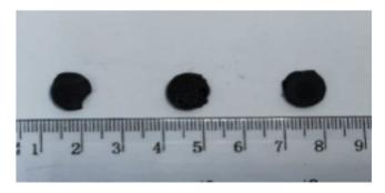
**Figure 2.** Discs of PDMS:Fe<sub>3</sub>O<sub>4</sub> composites obtained by free polymerization (left and right) and magnetic polymerizations (middle).
