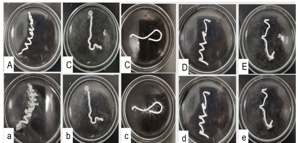
Figure 7. Anti-washout properties of the composite bone cement with different PLGA-PEG-PLGA temperature-sensitive hydrogel contents: (A–E) photos of as-prepared 0, 10, 20, 30, and 40% v/v PLGA-PEG-PLGA/C 3 S/C 2 S/POP bone cement slurry injected into SBF solution at 37 °C, respectively; (a–e) corresponding photos after shaking using a horizontal rotary oscillator for 1 min.
