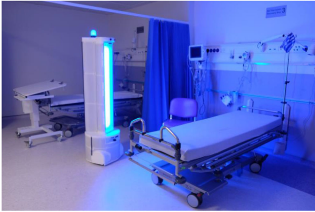
FIGURE 1 Example of a robotic UVGI platform being used to disinfect surfaces in a hospital
